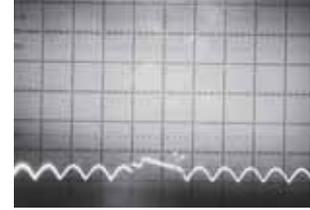
RIGHT: When transient protection circuitry is added to the DC output, the 1400 volt transients are leveled to a safe 250. (These tests were conducted with a Tektronix 535 oscilloscope with 10-to-1 attenuated probe.)
