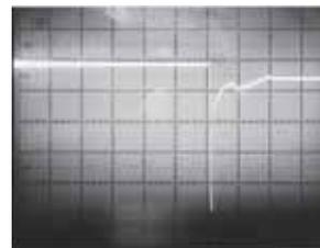
LEFT: Typical trace with capacitor as coil suppressor when 28 volt pulse to inductive load is interrupted. Collapsing magnetic field can generate a spike in excess of 350 volts. Spikes can short capacitors, cause coil burnout or damage other circuit components.
