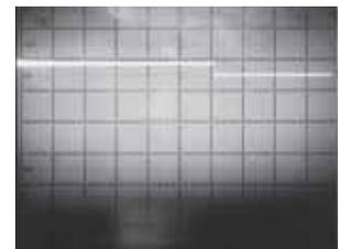
RIGHT: Same inductive load interrupted under identical conditions, but with coil suppressor No. 122654-001 connected in parallel with coil. Results:
