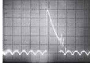
LEFT: Actual wave form read from DC output of unprotected full wave silicon bridge rectifier powering an inductive load. To prevent cell destruction, 1500 PIV (IN-1150) diodes were used. Typical DC output of bridge appears between 0 and 165 volts.
